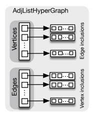
Fig. 2: Adjacency list hypergraph data structure.
